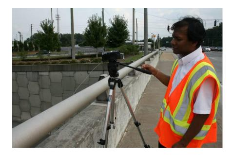
Figure 18: Camera Assembly Height Camera and Tripod are Tethered to the Rail
