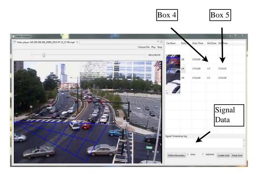
Figure 21: Creating exit zones and exit time stamps in VideoAnalyzer.
