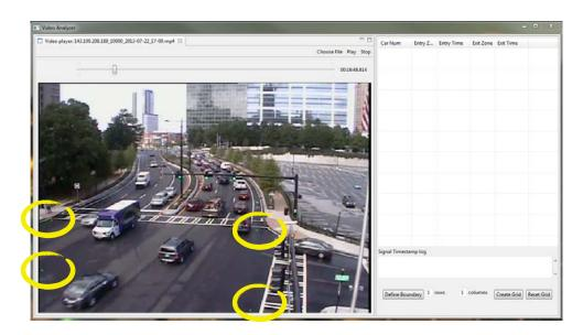
Figure 18: Selecting grid boundary points in Video Analyzer.
