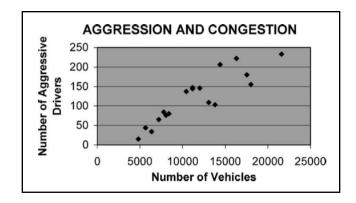
Figure 1: The number of aggressive drivers observed as a function number of vehicles on the road in the same direction of travel (4 hr period) (17).
