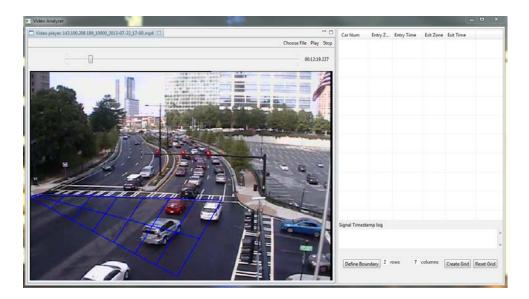
Figure 19: Grid created in VideoAnalyzer.
