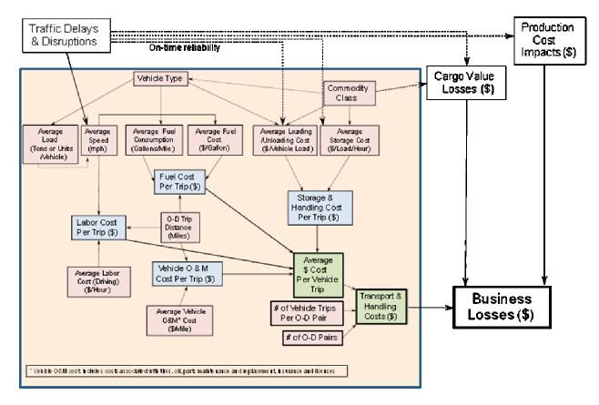
Figure Fourteen: Flow chart of model components for future research
