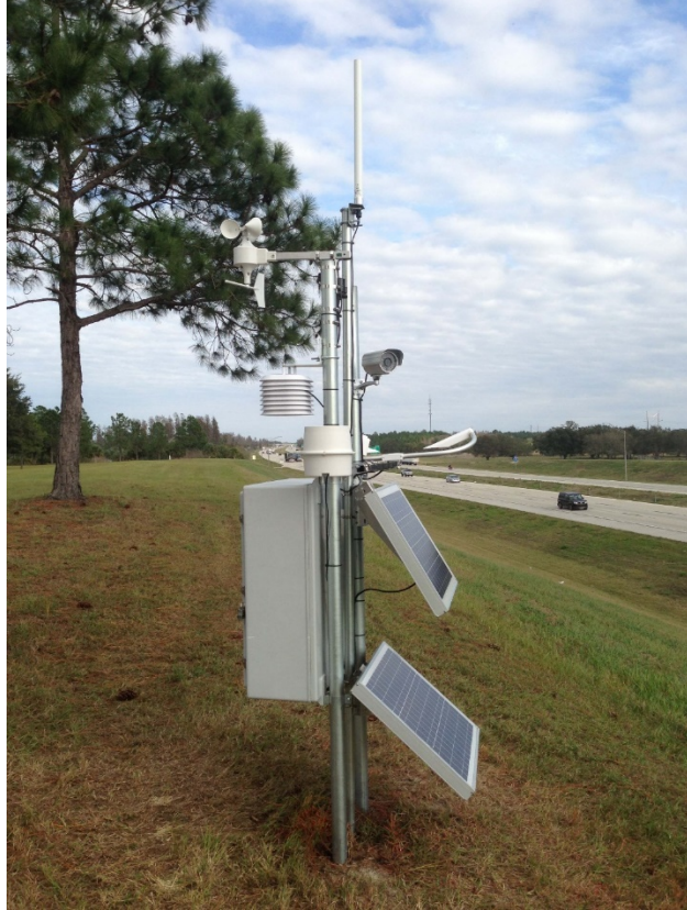
Figure 3-4 Camera, visibility sensor, and meteorological sensor stack
