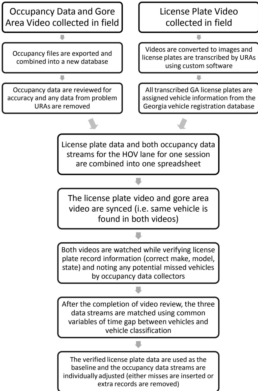
**Figure 6: Flow Chart of Matching Process**
