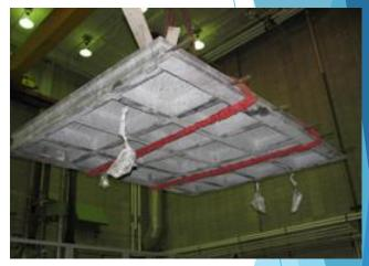
Images taken from full scale laboratory test of UHPC waffle slab bridge deck for Wapello County, Iowa
