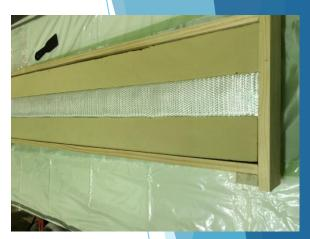
Installing foam and laying shear fiber
