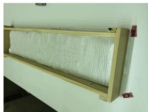
Putting the side mold and laying the top glass fiber sheets
