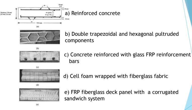
Tests conducted by Alagusundaramoorthy et. al. on four different FRP panels by criteria of the Ohio DOT using reinforced concrete as a baseline.
