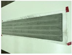
Laying the peel ply, infusion mesh, and UHPC plate
