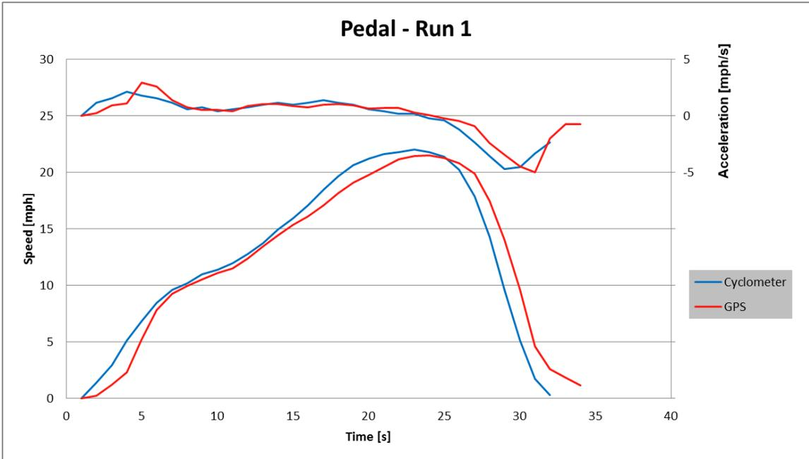
**Figure 77. Lab Test Speed and Acceleration – Pedal 1**
