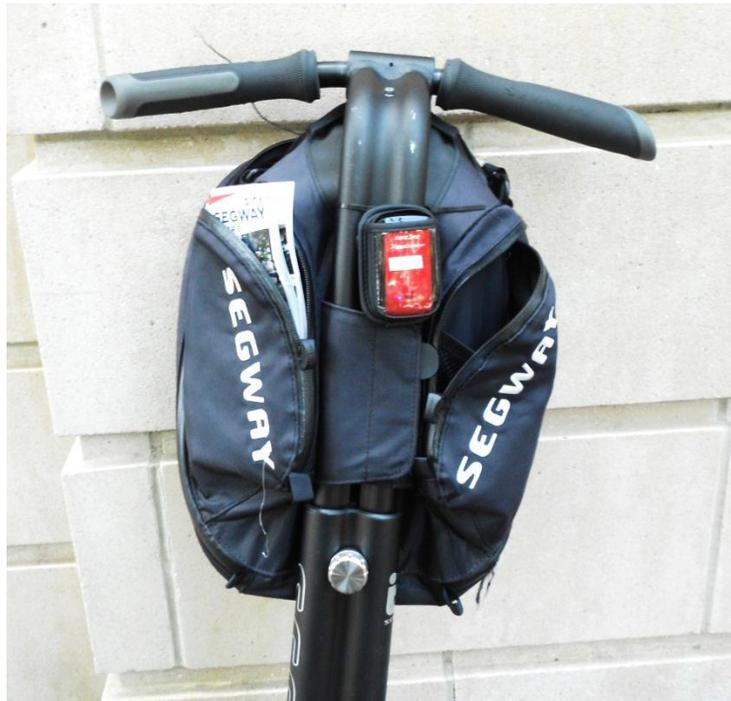
**Figure 32. GPS recorder Instrumented on Segway**
