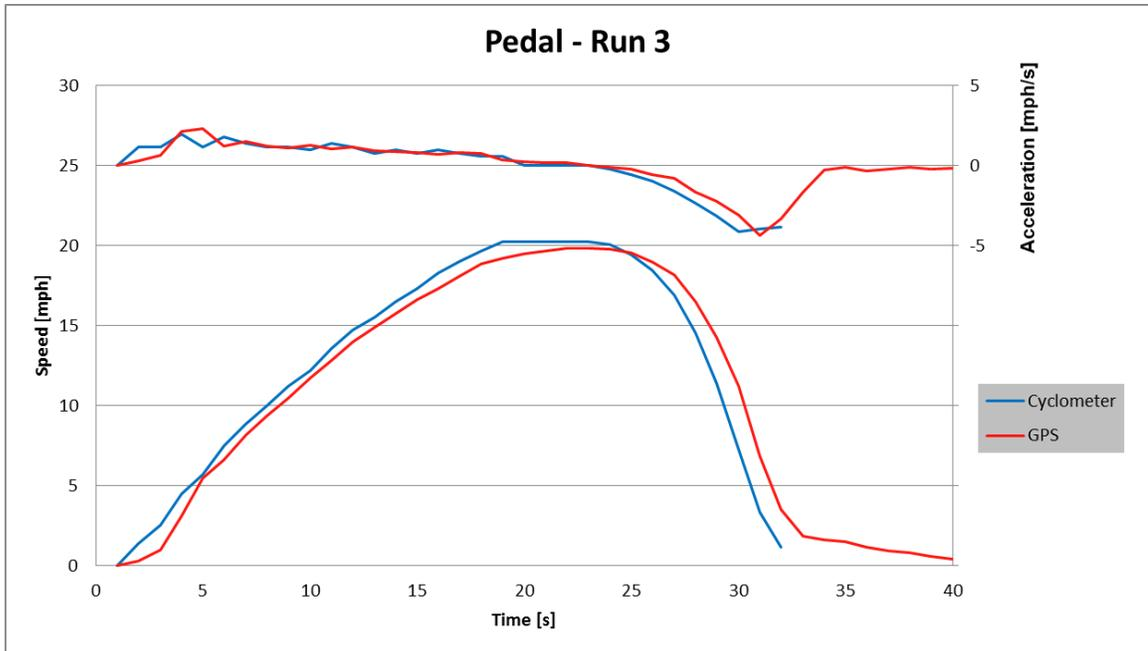
**Figure 79. Lab Test Speed and Acceleration – Pedal 3**
