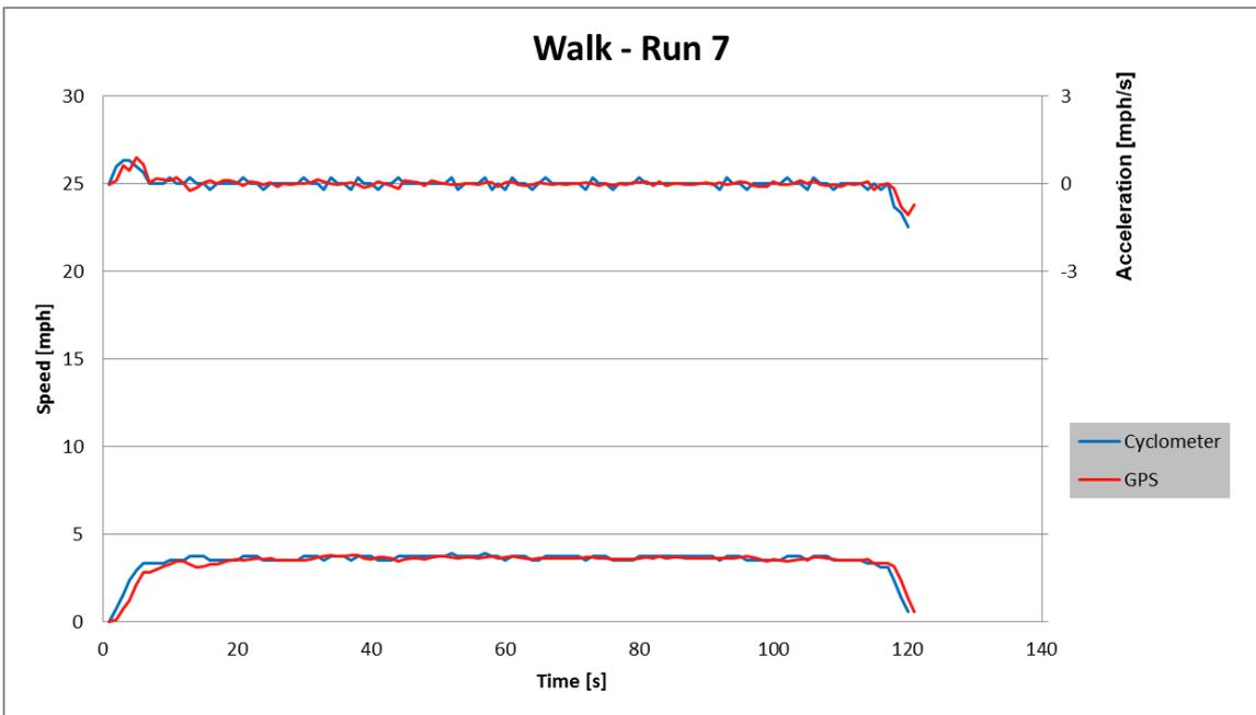
**Figure 63. Lab Test Speed and Acceleration – Walk 7**
