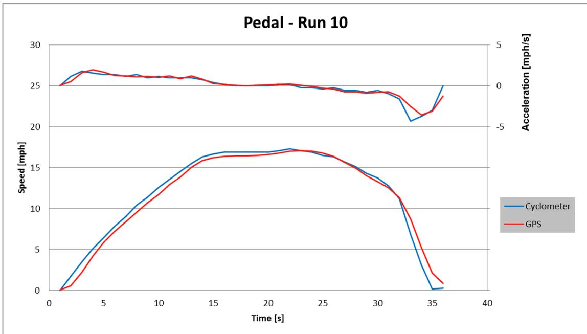
**Figure 86. Lab Test Speed and Acceleration – Pedal 10**
