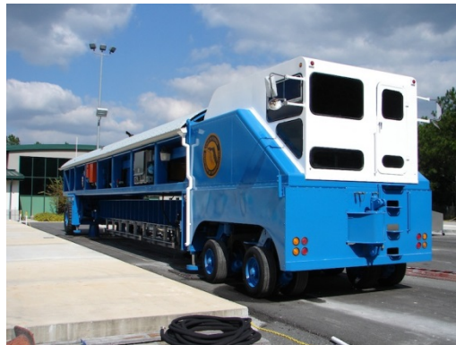
Accelerated Pavement Testing Vehicle in Gainesville, FL (courtesy FDOT)
