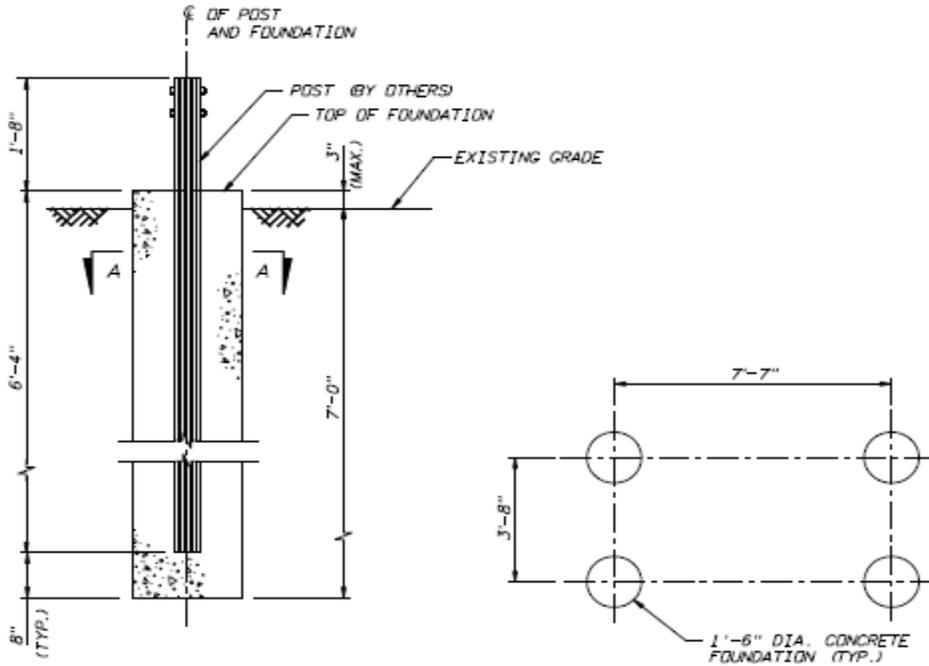
CONCRETE FOUNDATION ELEVATION
