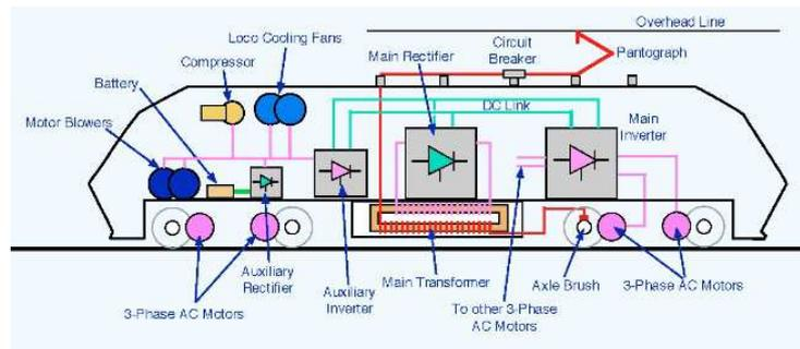
**Figure 21: Electric locomotive parts**
