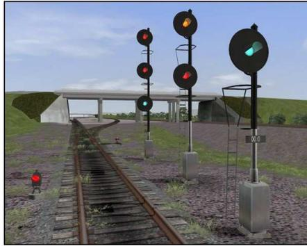
**Figure 15: Conventional track side signaling system<sup>14</sup>**
