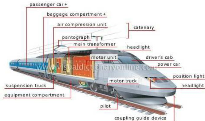
**Figure 19: High speed trains components**
